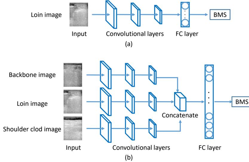
Figure 6. (a) Network architecture based on general knowledge. (b) Network architecture based on Knowledge 1, revealed by our field survey. Here, “FC” means “fully connected.”
