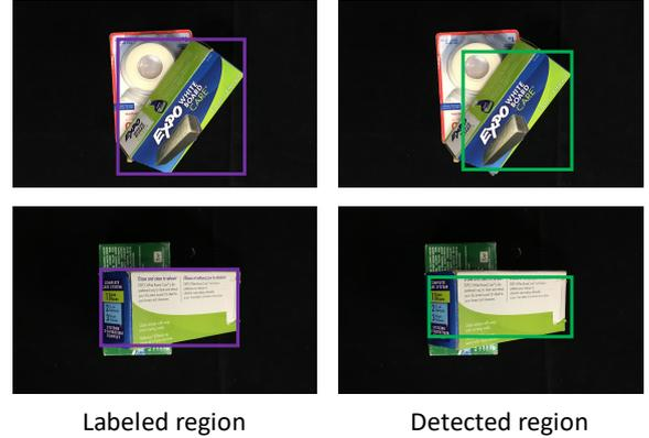
Fig.15 Example of detected region and labeled region. The purple box represents labeled region. The green box represents detected region.
