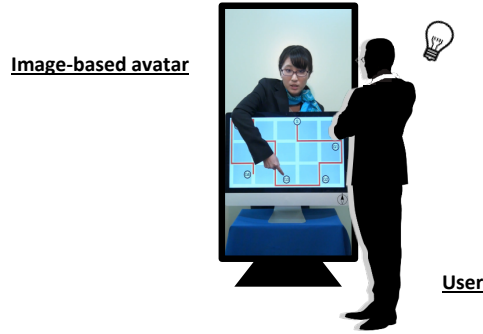
Fig. 1. Route navigation system that uses an image-based avatar that points at a map.
