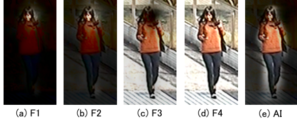
Fig. 5. Examples of pedestrian images after applying correction functions. We used the gaze map in (a) to (d) and the average intensities in (e)
