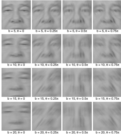
Fig. 11. Examples of synthesized images of camera motion blur from the subset ‘fb’ of FERET. Blurred images are synthesized from Figure 6 (a) using linear motion blur PSFs with given b, \theta .
