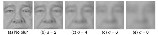
Fig. 6. Examples of synthesized images of camera focus blur from the subset ‘fb’ of FERET. Blurred images (b), (c), (d), and (e) are synthesized from the original image (a) using Gaussian PSFs with given standard deviations \sigma .
